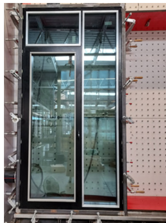
Test stand for testing parameters of curtain walls, windows and doors
