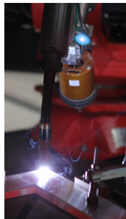
Welding of aluminium
